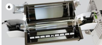
Before placing the new lamp, make sure the contact wire is straight, the getter is on the ballast side and the text on the lamp is facing out.
