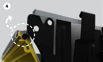
Pry open reflector edge from casing using a spudger tool
