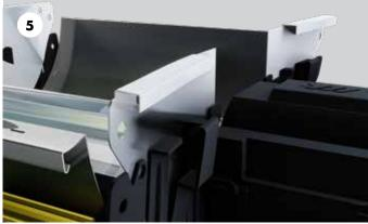
Lift reflector up and remove
