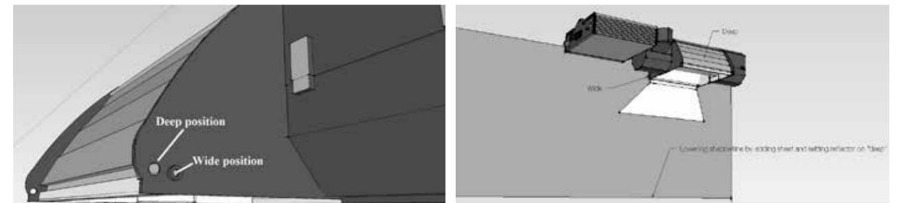
When the side-reflector is moved to the outer position, the reflector is in "deep" position, when moving the side-reflector towards the lamp the reflector is in "wide" position.
