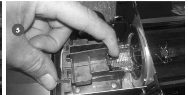
Slide fittings on both sides away from the lamp and lift out lamp
