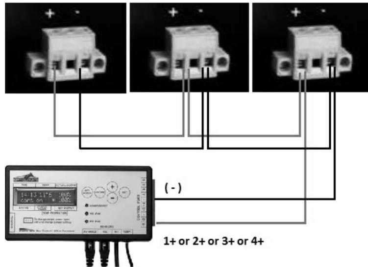
The Maxi Controller sends a signal to the fixtures to switch them on or off. There are 4 ports on the Maxi controller, each port can switch up to 40 fixtures. To connect the signal wire from the controller to the first fixture and looping it to the next, we suggest to use a black/red wire (speaker cable) so + and - are not mixed up.
